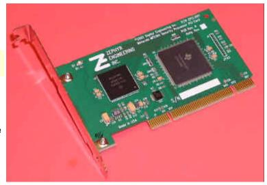
The **ZPCI.3911** MPC184 Security Processor PCI card from Zephyr Engineering, Inc is a high-performance encryption/decryption engine on a universal (5V/3.3V) 32-bit 66 MHz PCI card.
